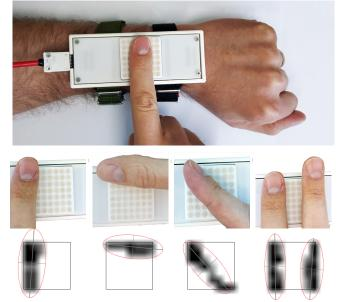
Figure 1. Top shows wearable prototype – the raised central square is the sensor. Bottom image pairs show area touches (index, thumb, side of index and index and middle fingers) and corresponding sensor activations.
