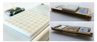
Figure 3. Left image shows close up of 33m square sensor area standing 3mm proud of the surrounding surface. Darker circles are the touch sensor electrodes. Right two images show the device outside its casing from top (upper image) and bottom (lower image).
