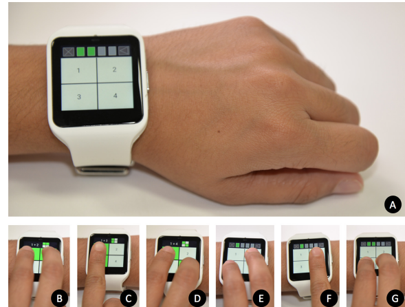
Figure 1: PIC Unlock Screen. Top image (A) shows a PIC unlock screen on a smartwatch running the interface from study 3. PICs are a chorded input system composed of four single-tap inputs achieved by selecting the keys labeled 1 to 4, and six dual-taps inputs achieved by selecting any pair of these keys as shown in figures B through G. Dual-taps can be entered with either two fingers (B, D, E, G) or a finger placed flat over two keys (C, E).
