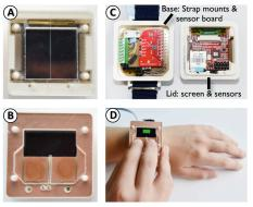
Figure 1. Watch prototype created for study. Plan views of watch screen with transparent ITO sensors (A) and halfscreen PCB sensors (B). Right images show internal structure (C) and PCB prototype mounted on user's wrist with fingers touching the sensors and screen showing study UI (D).
